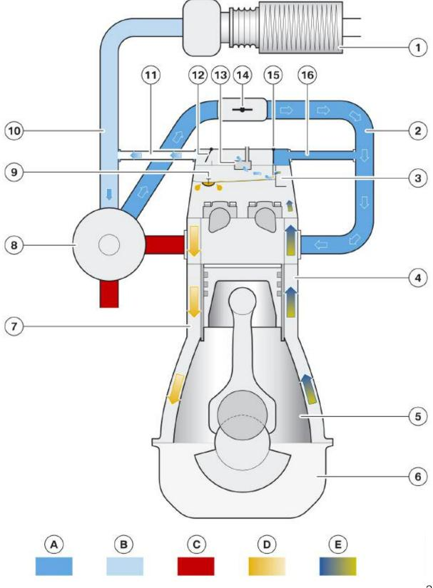
N55, crankcase ventilation, turbocharged (boost) mode
